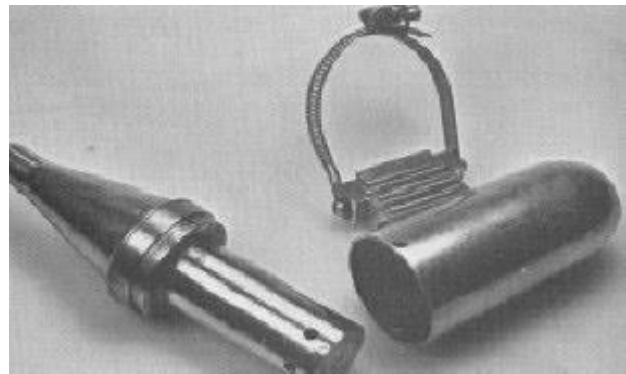
Right: the inside of the current Webra 1100/E-G6 silencer. See text for details. (Redshift 60 tested).
